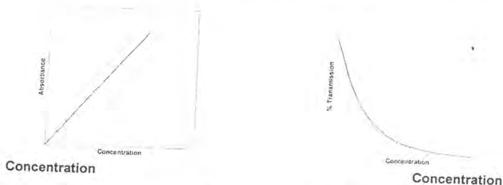
Figure 3: Beer-Lambert Law relates the amount of light Absorbance (A) by a solution to the Concentration (C) of a compound in solution and the length of light path:
