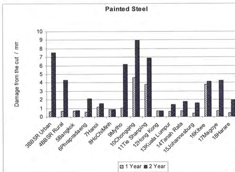
Figure 2.23 Degradation of painted steel after 1 and 2 years of exposure at CORNET sites across Asia and southern Africa.
