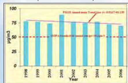
Decreasing trend of Annual averages of PM at Colombo Fort Ambient Air Quality Monitoring Station (1998-2006)
