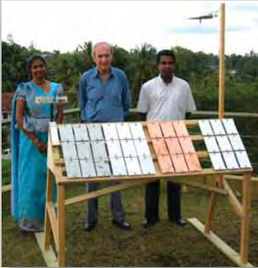
Corrosion Rack at CEA office, Sri Lanka
