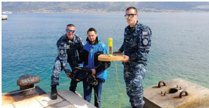
Deployment of AUV D2 with an integrated forward looking sonar.
