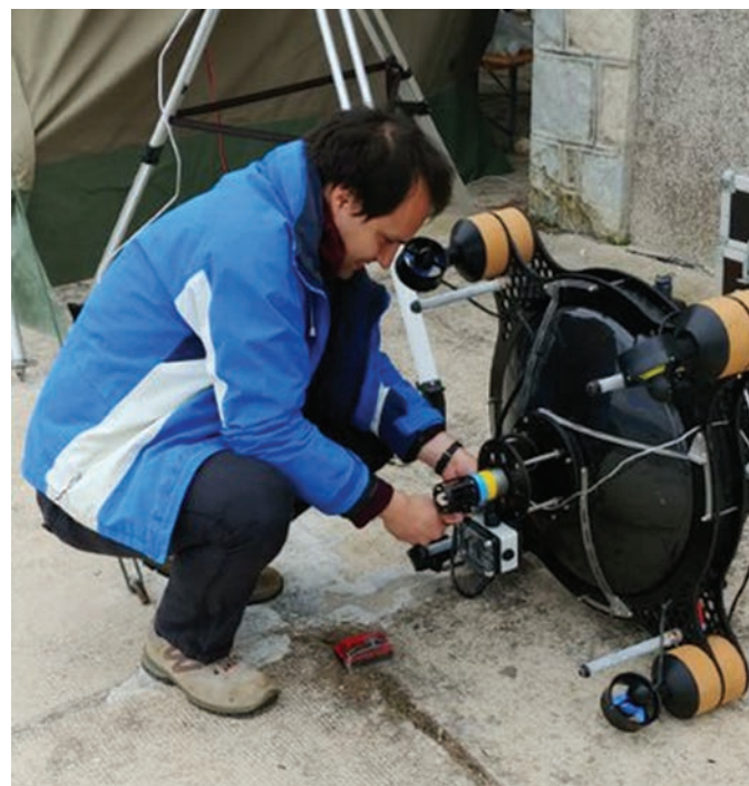
ASV Proteus with mounted SeaTrac USBL and downward looking camera.
