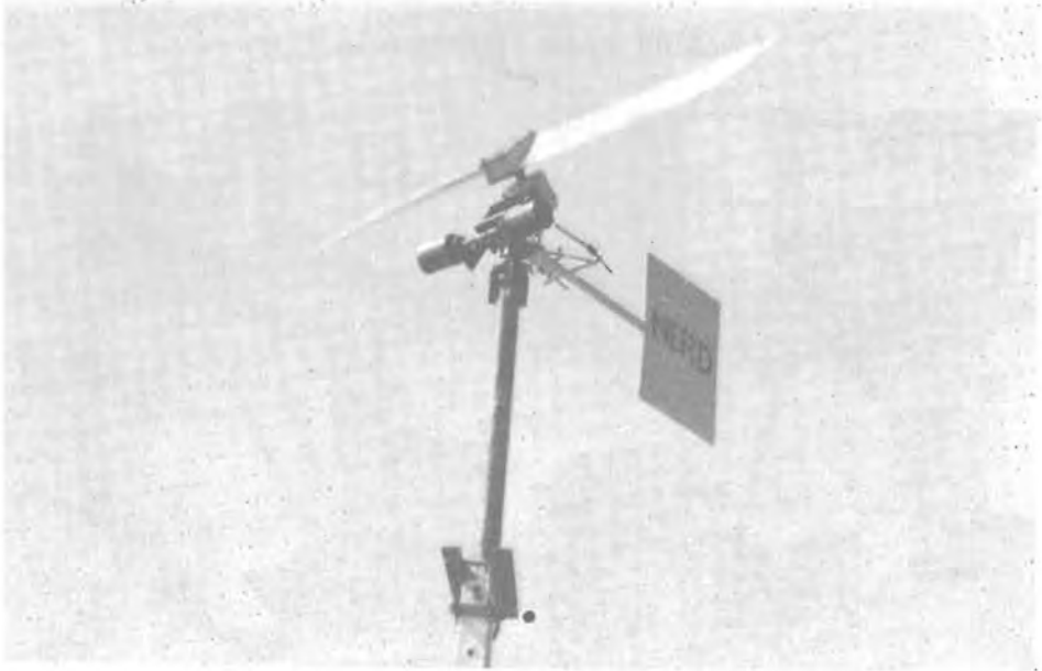
Windmill generator and battery charger together with windmill powered Air compressor
