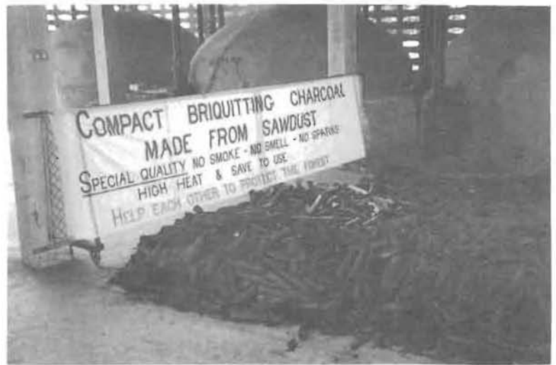
Charcoal produced from sawdust briquettes in Northern Thailand A new market for "wood waste"
