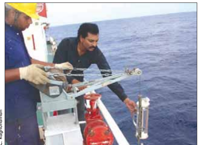
Using a Nansen seawater collection bottle for oceanic monitoring in India
