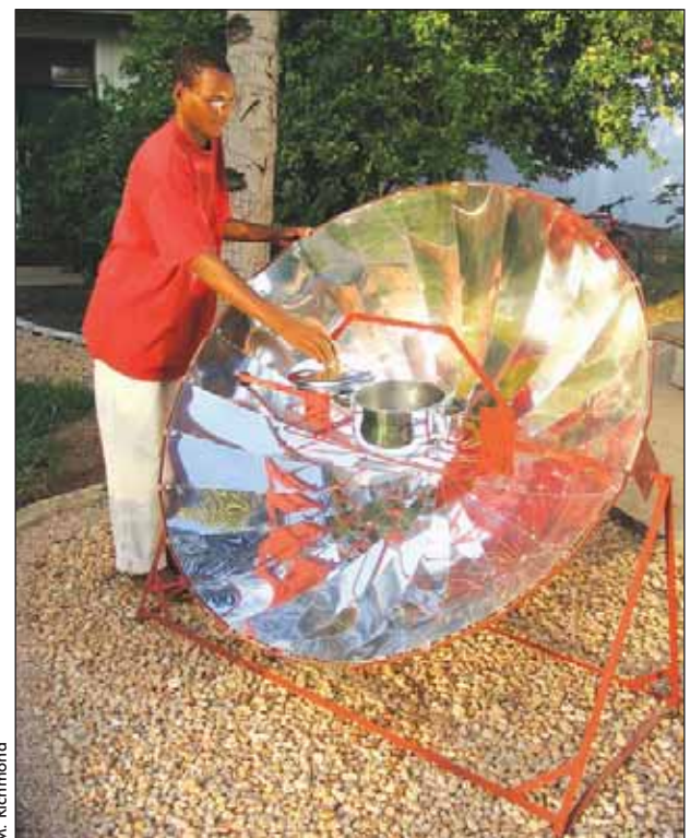
Solar cooker being used to boil water
