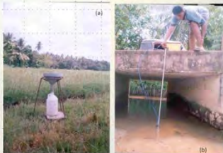
(a) Rain Gauge ( R_1 ) installed at the paddy field; (b) water velocity and stage measurement at culvert mouth using current meter
