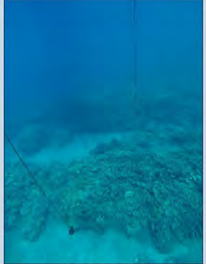
The particle motion accelerometer hangs in the background while an acoustic listening device hangs in the foreground. The accelerometer is suspended from a mooring that was specially designed to isolate movement. (Photo by T. Aran Mooney, Woods Hole Oceanographic Institution)
