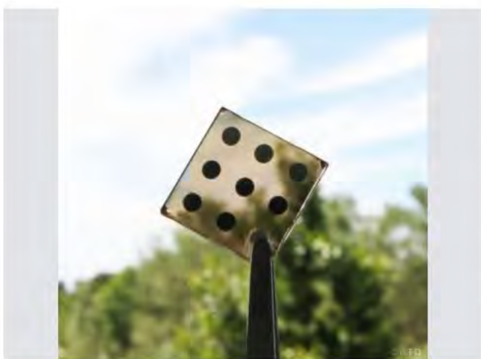
This image shows a semi-transparent solar cell based on AgBiS2 nanocrystals. Credit: ICFO
