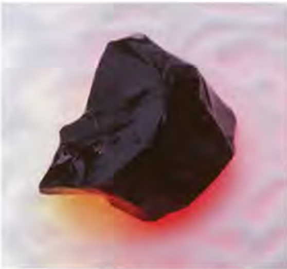
Photo: Albert Kruger/U.S. Department of Energy Glass produced from a high level radioactive waste simulant.
