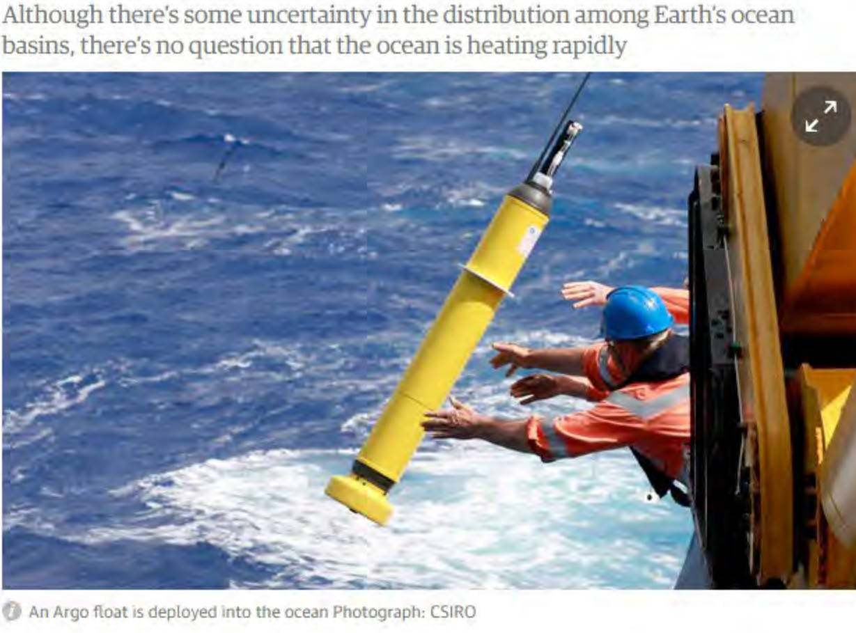
An Argo float is deployed into the ocean Photograph: CSIRO
