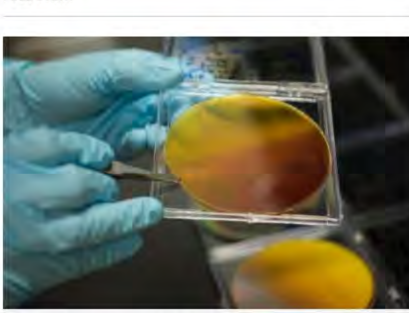
New materials are created through deposition onto disks, which are then tested to determine their properties.
