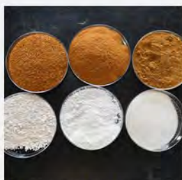
Researchers at The Ohio State University have developed a patent-pending technology for incorporating food waste into rubber. Here, dried and ground tomato skins (top) and eggshells (bottom) are shown after coarse, medium, and fine processing before being added to rubber. Photo by Kenneth Chamberlain, courtesy of The Ohio State University. - Download
