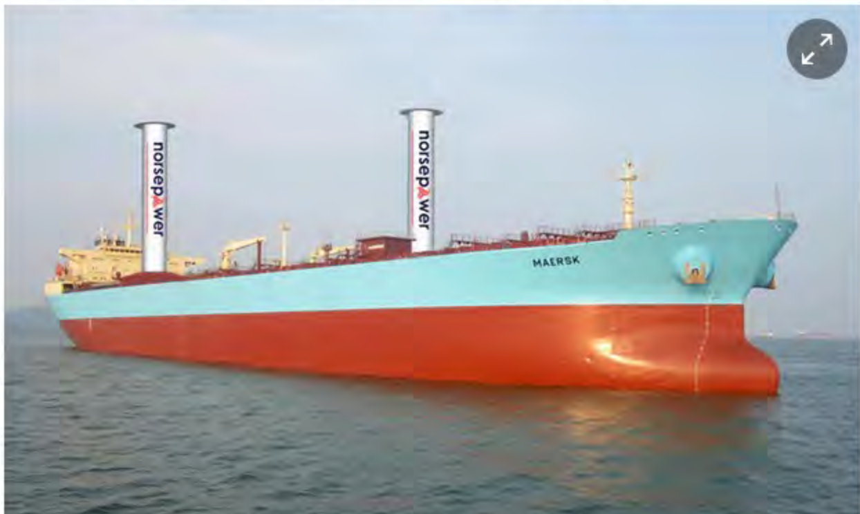
The Maersk container ship fitted with Norsepower rotor sails. The technology was first invented by the German engineer Anton Flettner which he trialled on an Atlantic crossing in 1926. Photograph: Courtesy of Norsepower
