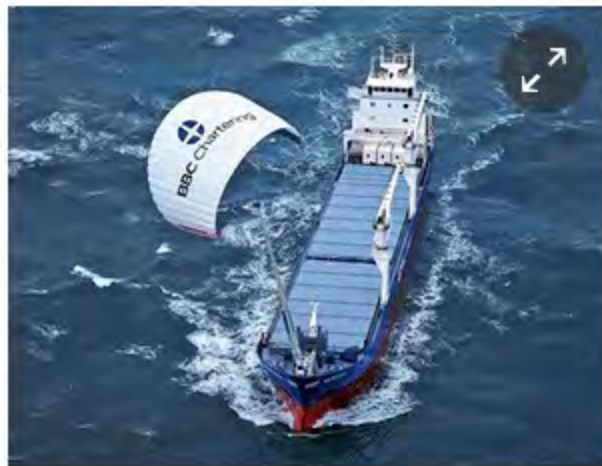
The German company SkySails uses large kites to provide wind power to reduce fuel costs and emissions. Photograph: SkySails GmbH
