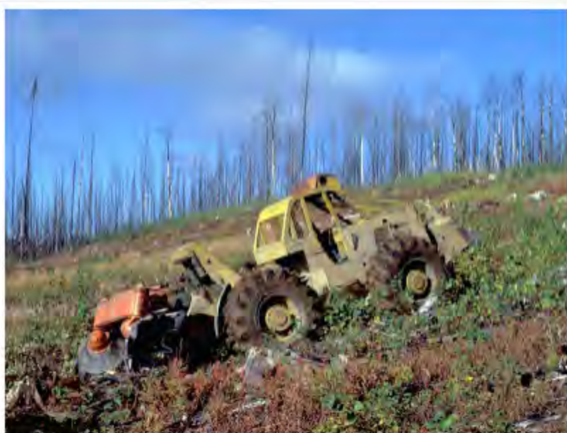
A disk trencher removes vegetation in the slope unit in 1985.
